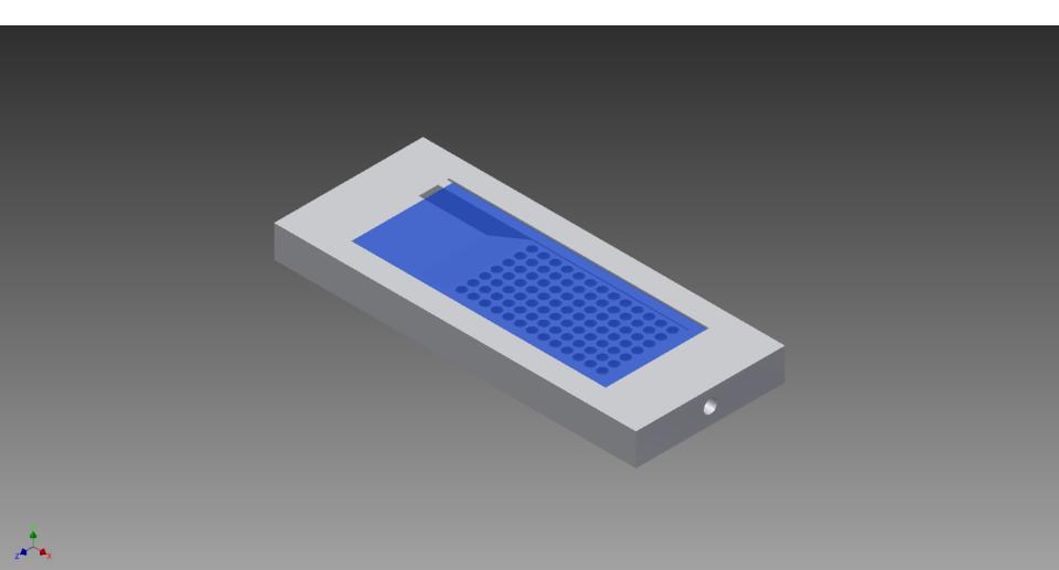
Fully assembled device included sealed coverslip (shaded blue) and sealed microscope slide (shaded green).
